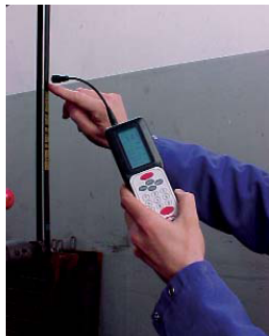
TENSION CONTROL BY VIBRATION METHOD
